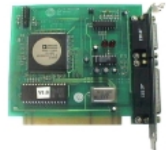
SHARC-based demodulator fitted in half-sized PC card
