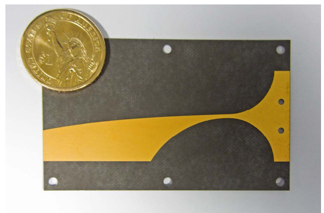
Figure 1. Bottom layer of the final tapered-slot antenna design
