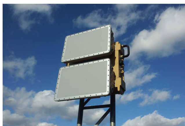
Figure 6. Two 5^\circ beamwidth antennas deployed on radar
