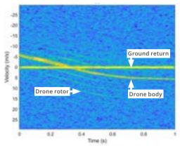
Spectrogram of raw radar data showing return from the ground and from a drone, which approaches then receeds from the radar.
