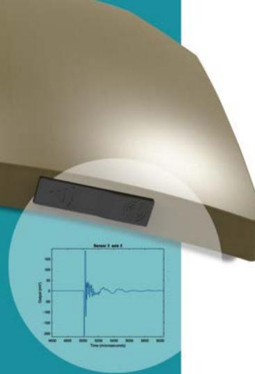
Example signature measured by a ceramic armour monitoring device that can identify the signal characteristics associated with crack formation following an impact event.
