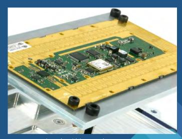
mm-wave scanning radar with integrated antenna
