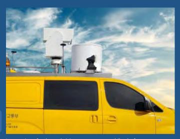
Integration of radar and vision system on a mobile platform
