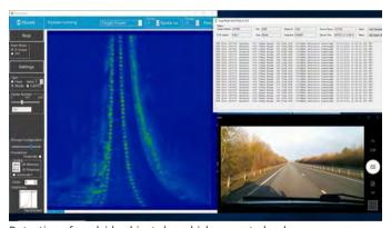
Detection of roadside objects by vehicle-mounted radar
