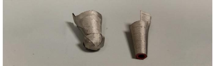
**Fig. 5. Ultra-soft Silver-Aluminium silicone material around plastic ear-buds**
