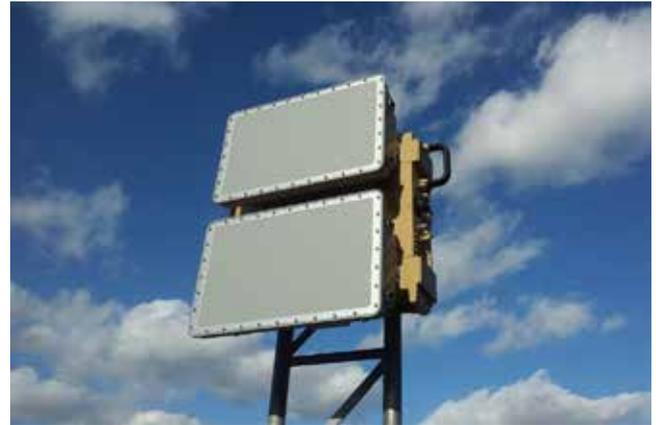
Figure 6. Two  $5^\circ$  beamwidth antennas deployed on radar
